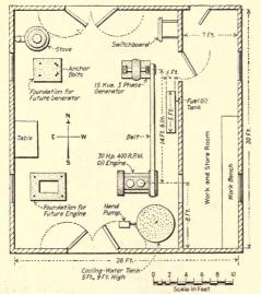
Fig. 283.—General lay-out of small oil-engine plant.
